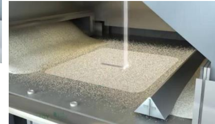
Energy is brought by the Electron beam to melt the particles
