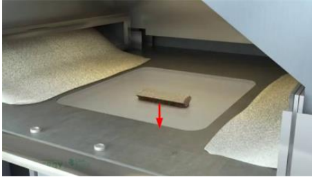
The building tray is moved down
